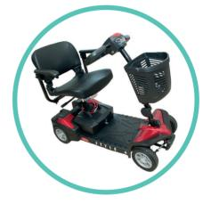
• 'class 3 invalid carriages' These can be used on the road, and have a maximum speed of 4mph off the road, and 8mph on the road.
